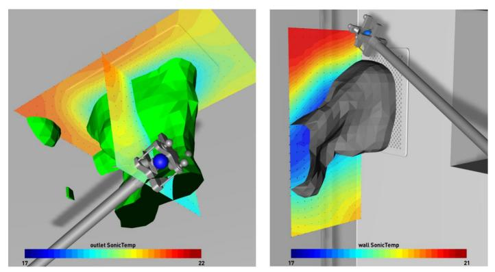
Ceiling (left) and wall outlet showing the airstream (green iso-surface at 0.15 m/s and gray at 0.2 m/s) entering at 3-4°C below room temperature and drop due to the higher density.
