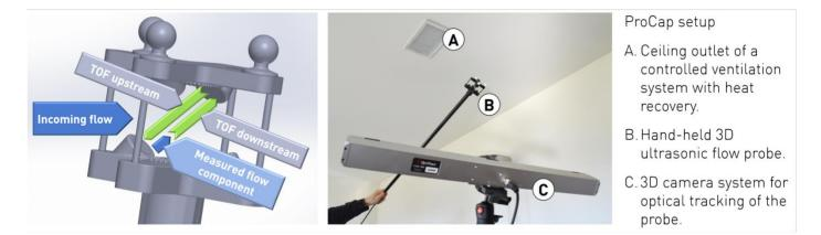
The TriSonica<sup>™</sup> Mini sensor from Anemoment uses two pairs of transducers with 4 possible paths and can measure all 3 components of the flow (with some restrictions to the acceptance angle due to the structure). Additional sensors for ambient pressure, temperature and humidity are fitted and allow to calculate the fluid density.
