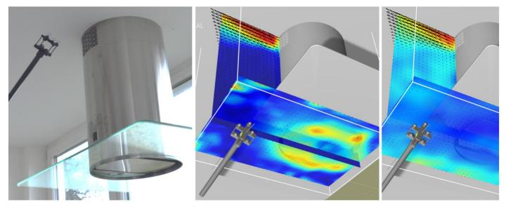
Flow around a recirculating cooker hood (left). The flow at the inlet (center) is one order of magnitude slower (max. 0.8 m/s) than the outlet at the top (8 m/s). The temperature (right) shows an increase of 3°C due to the losses in the fan.
